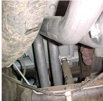
Install passenger side over axle tailpipe # C into muffler and attach using clamp # G. Insert welded hanger into rubber grommet. Use bolt kit # H to attach the tailpipes together. Do not tighten. **YOU MAY NEED TO LOOSEN YOUR SPARE TIRE & PUSH TOWRDS DRIVER SIDE & RE-TIGHTEN**
