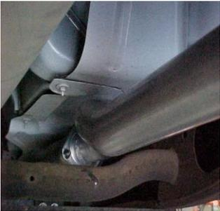
Install head pipe # A onto your existing stock flange re-using the factory hardware. Use a jack stand to support the converter. Do not tighten. Insert welded hanger into rubber grommet.
